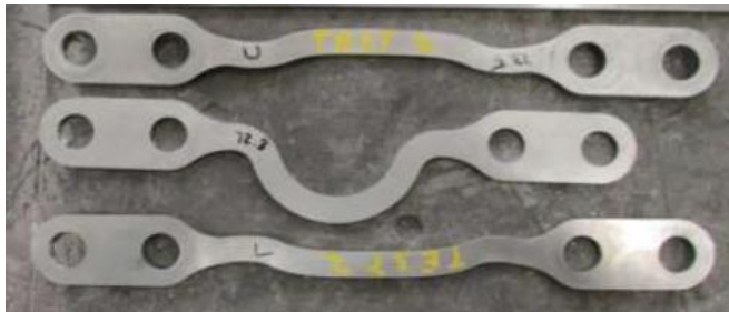
Figure 14: Scaled double c-dampers pre and post-test
