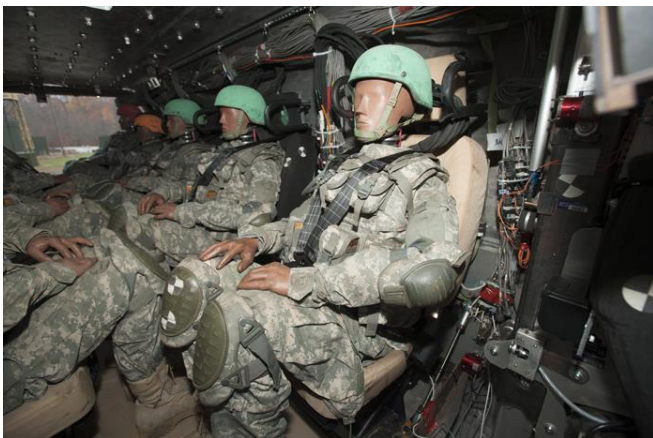
Figure 36: Test asset with full ATD load
