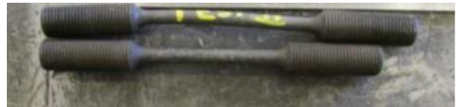
Figure 16: Scaled tension rods pre and post-test
